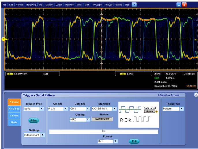
Serial pattern triggering to debug pattern-dependent issues.
